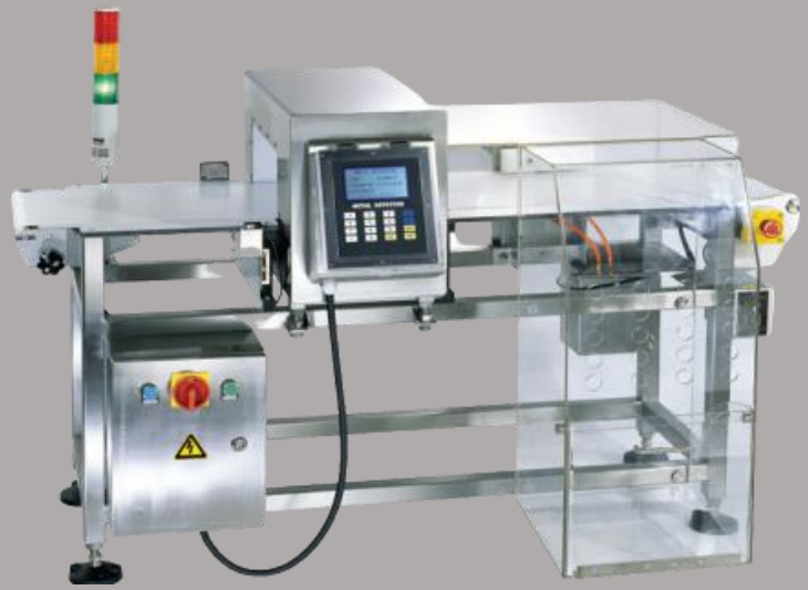
Metal detector (tests up to 100 pcs/min)
